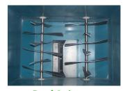
**Dual Agitators**Designed for Constant Material Flow
